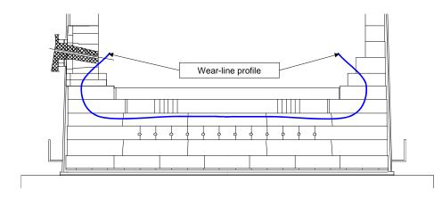
The location of the 1150°C isotherm is estimated solving a non-linear inverse heat transfer problem, where the observations are temperature measurements and the unknown is the geometry.
