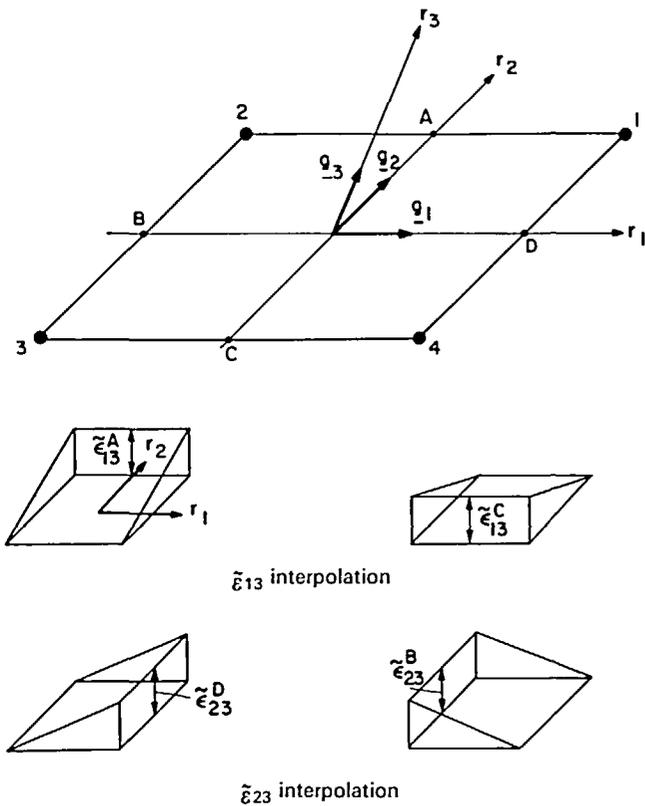
Figure 2 Interpolation functions for the transverse shear strains
