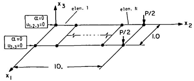
(a) Cantilever subjected to transverse tip load
