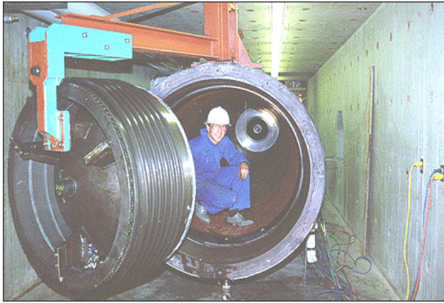
Figure 3. C-FER Deepwater Collapse Chamber
