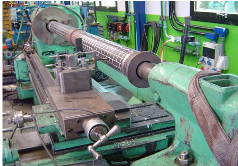
Figure A.1: The IMS (or shapemeter)
