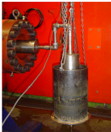
Figure 4.6: Internal Volume Variation Measuring System
