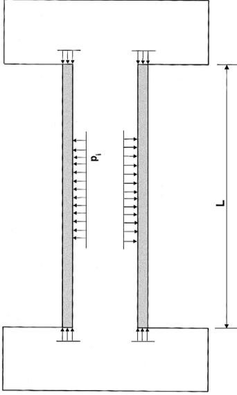
Fig. 2. Simply supported pipe open on both ends under internal pressure.
