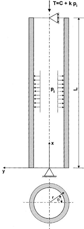
Fig. 1. Cylindrical pipe under internal pressure and axial compression.
