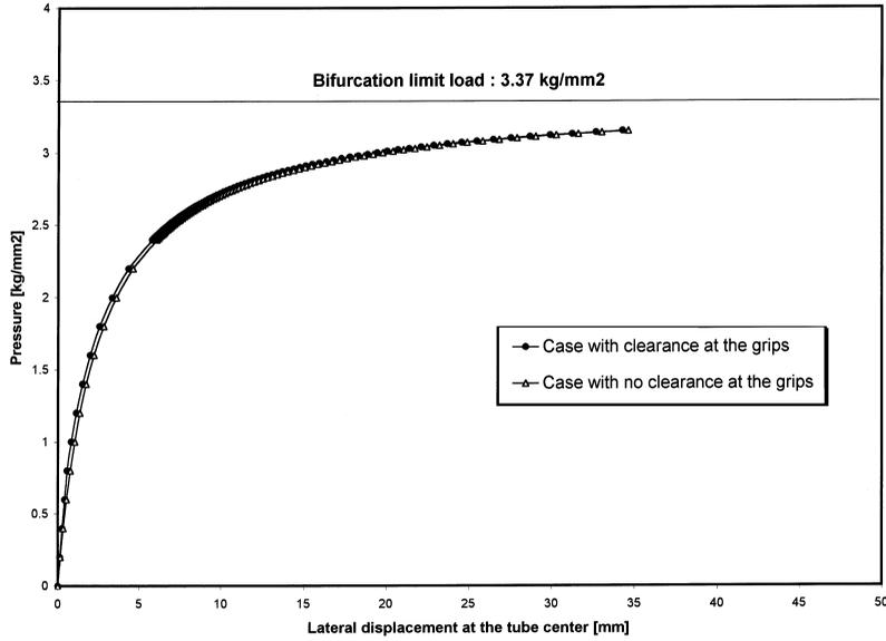
Fig. 4. Clearance between grips and pipe body. Load–displacement curves.
