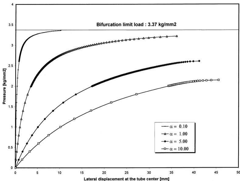
Fig. 3. Grips with no clearance. Load–displacement curves.
