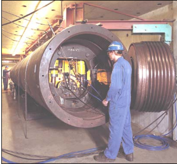
Figure 3. C-FER Deepwater Collapse Chamber
